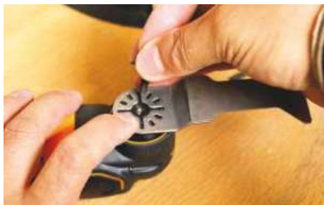
▲ Standard cutters need to have the retaining screw fully removed to swap them
